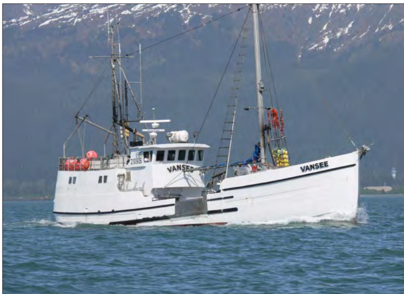
A halibut schooner slices through the waves at an efficient travel speed, as evidenced by the small bow and stern waves.
