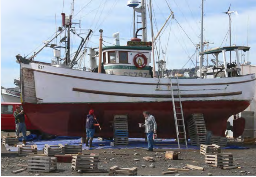
Renewing bottom paint on this classic troller prevents fuel-robbing bottom growth from taking hold.
