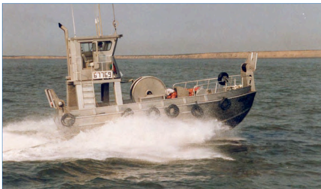
This planing gillnetter uses a lot of fuel per mile traveled, but its efficiency may actually be better at this speed than a few knots slower.
