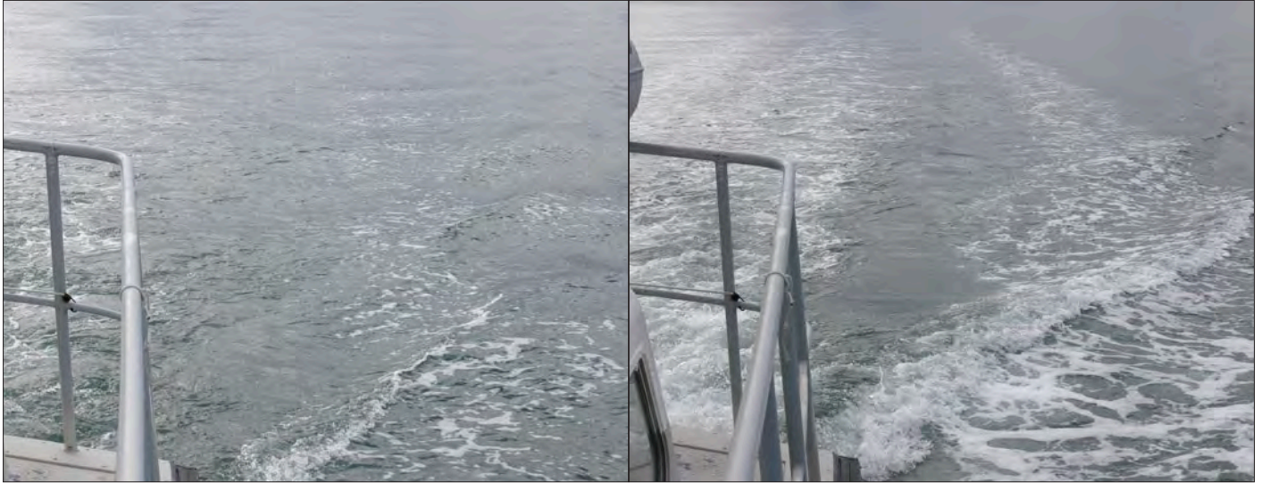
Two photos illustrate the difference in stern wave of a 40 foot boat between 7 knots (left) and 8 knots. The bigger the stern wave the more power and fuel it takes.
