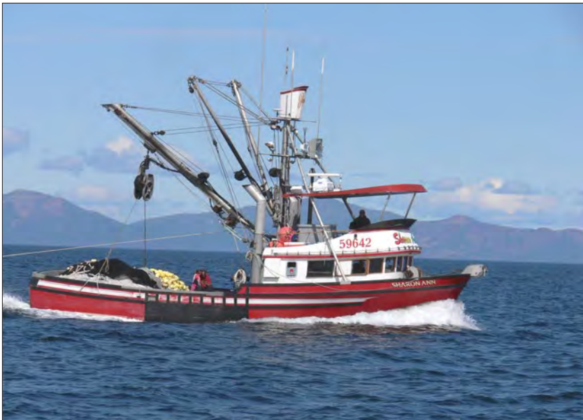
A seiner is steaming at about hull speed. The "bone in its teeth" shows that it is using more fuel than necessary.
